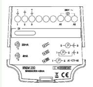
The sensor is preset from factory for a reading of 4-20 mA between the margins (D). If you want to calibrate again, connect it as shown in the diagram. Place the float at the bottom and set 4 mA in the instrument by the multiturn potentiometer [4mA]. Do the same with the potentiometer [20mA] placing the float on top.
