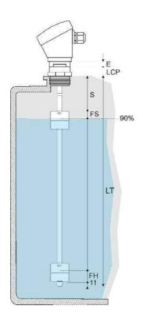
You can determine a height (S) to set an area where there is no reading at all. In case you want to remove the head of the connection process (for reasons of high temperature, for example) may specify a dimension (E) exceeding the standard.
